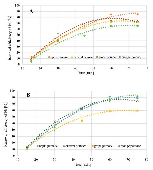
Figure 4. The efficiency of lead ions removal on fruit pomace: A - freeze-dried, B - conventionally dried
