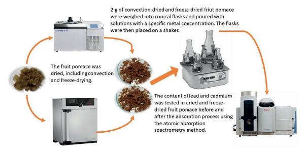
Figure 2. The scheme of performing the experiment
