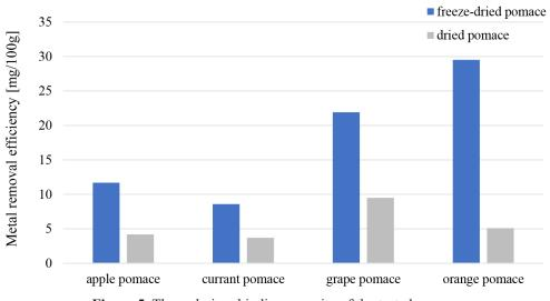
Figure 5. The cadmium binding capacity of the tested pomace
