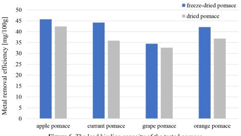
Figure 6. The lead binding capacity of the tested pomace
