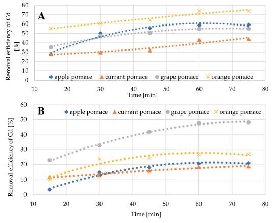
Figure 3. The efficiency of cadmium ion removal on fruit pomace: A - freeze-dried, B - conventionally dried
